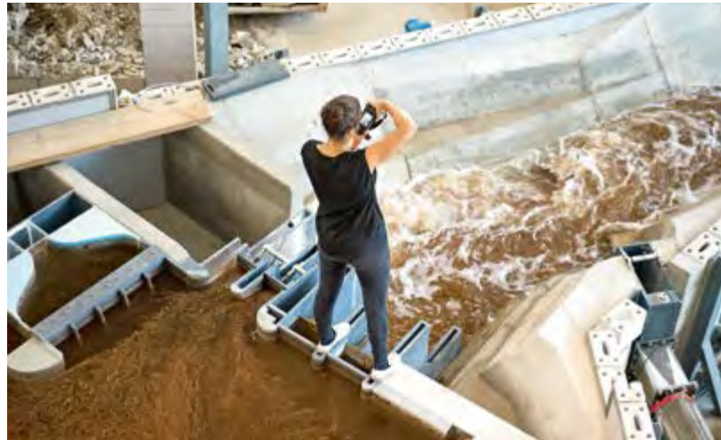
Claudia Beck documents the water flowing out of the reservoir. At the flood's height, the reservoir discharges 88 litres of water per second.
